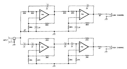
fig. 3. Schematic of the binaural synthesizer. For 750-Hz crossover, R = 21k; low channel is offset 5% high and high channel is offset 5% low to compensate for underlap due to four-pole cascade in each channel and overlap caused by approximately 4 dB of peaking on each side of the crossover point.
